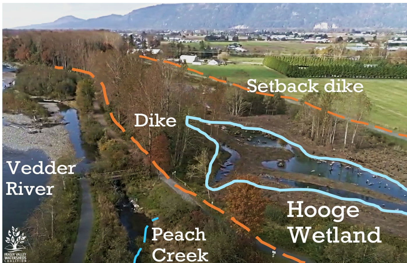
Figure 2: Hooke Wetland makes room for water by adding a setback dike, water can be stored between the dikes during high water flows. Photo Credit: Fraser Valley Watersheds Coalition
